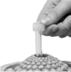
**Step 5:** Replace the silicone cap on to the extension tube.
